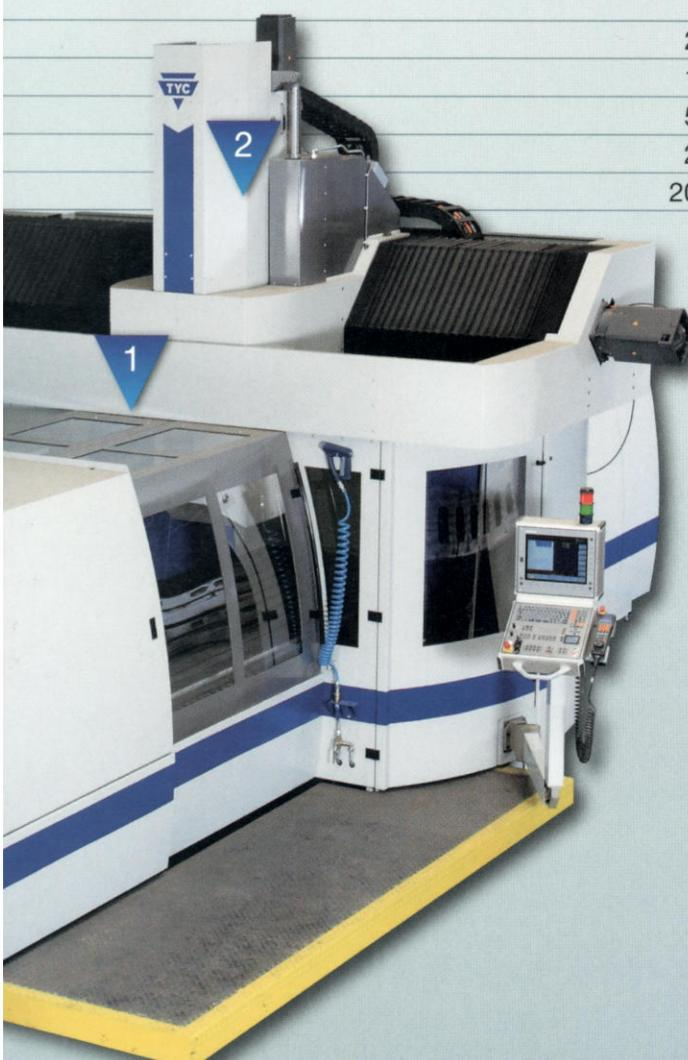
Portal type machining center FVC is designed as a very rigid machine, conception with travelling table and fixed frame.
